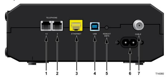
**Important:** Do not connect your PC to *both* the Ethernet and USB ports at the same time. Your modem will not function properly if both the Ethernet and USB ports are connected to your PC at the same time.
